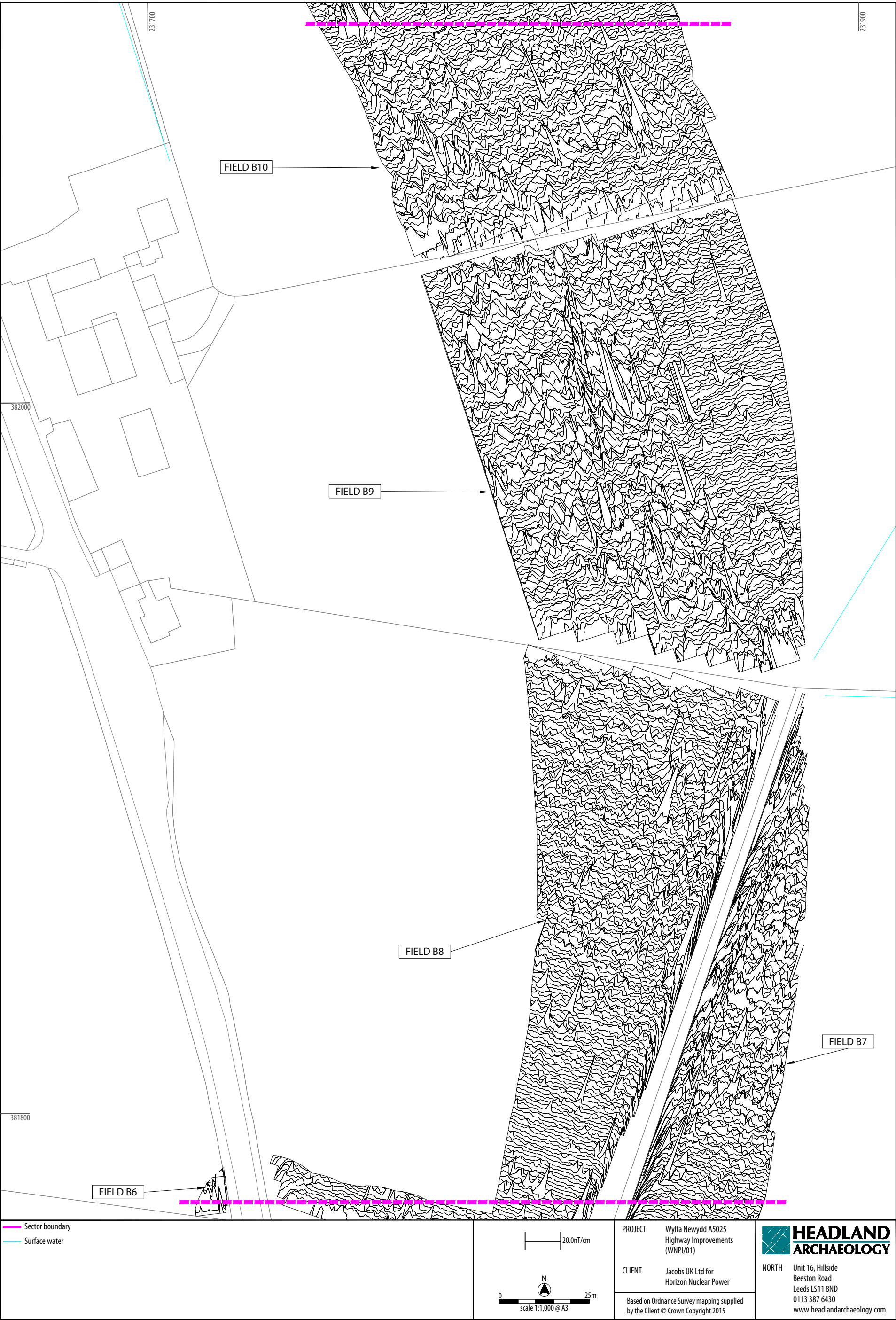
Illus 37 XY trace plot of minimally processed magnetometer data; Sector 5
