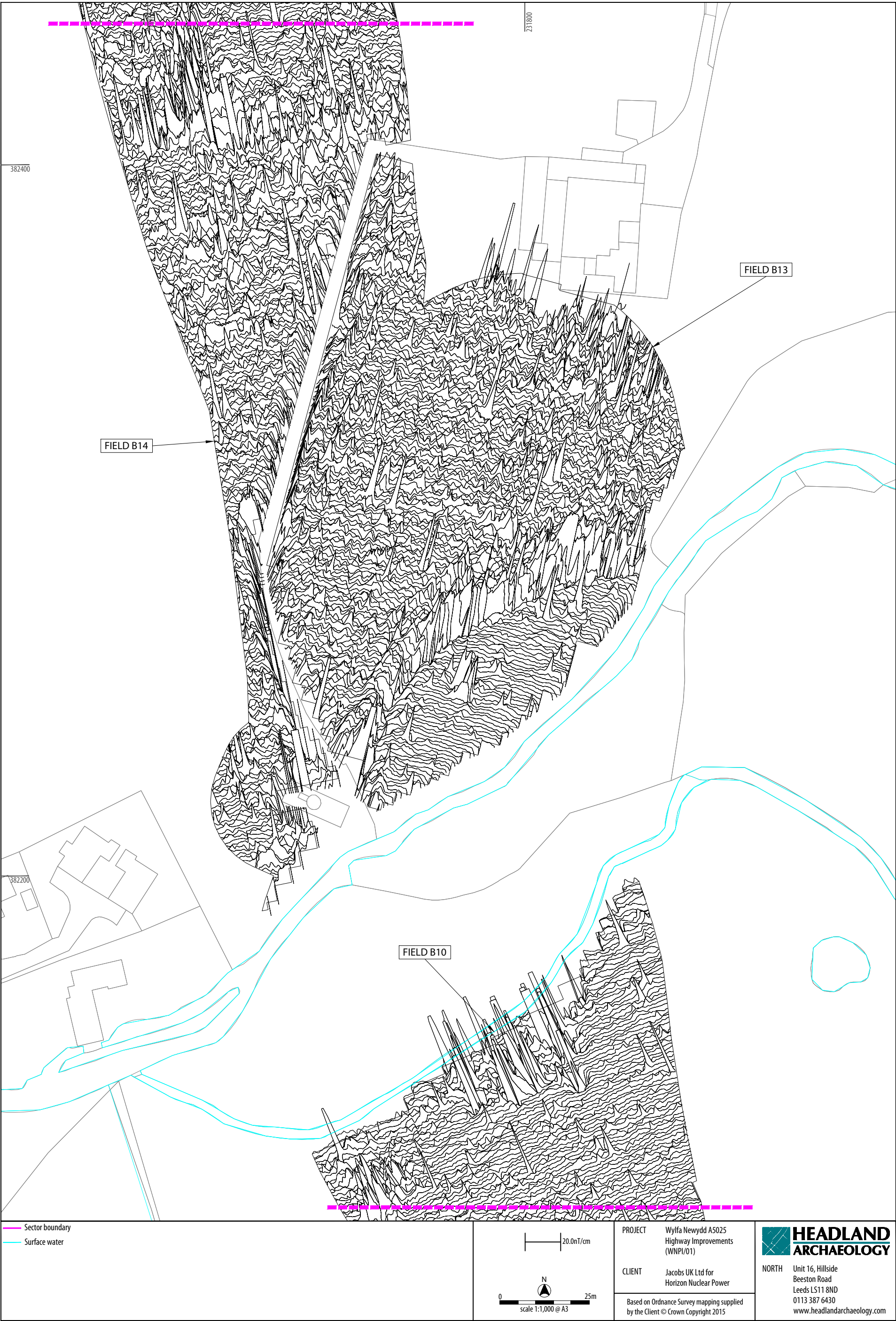
Illus 40 XY trace plot of minimally processed magnetometer data; Sector 7
